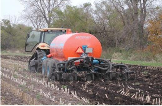
Slurry tank with injection toolbar for land applying slurry.
