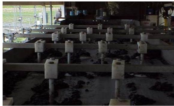
Suspended solids are separated using a gravity belt thickener and polymer
